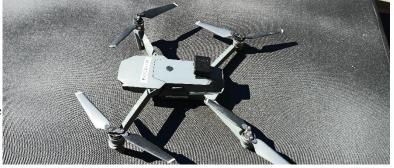
Pro because there's no way for me to tap into the batteries nor did I want to deal with attaching an RFID and a battery. You can see from the picture I just added some velcro to each of my battery packs and placed it there. Yes, it does affect the CG a little bit but the drone automatically adjusts for that.
